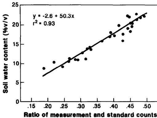
Fig. 3. Neutron probe calibration curve for the experimental vineyard. The line represents the linear regression fit between the ratio of measurement and standard counts and soilwater content (% v/v). SWC was determined gravimetrically and converted to v/v with the known sample volume.
