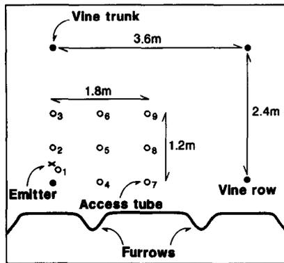
Fig. 2. Schematic diagram of vine and neutron probe access tube placement. Also shown are the positions of the emitter for drip irrigated vines and the furrows for surface irrigated vines.
