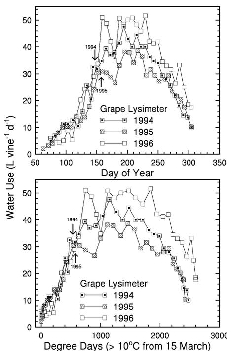
Fig. 3. Water use measured on Thompson Seedless grapevines grown in a weighing lysimeter for the 1994, 1995 and 1996 growing seasons as a function of day of year and degree-days from March 15. Each data point is the average daily value for a 7-day period. The arrows represent the approximate day the vines were girdled in 1994 and 1995.
