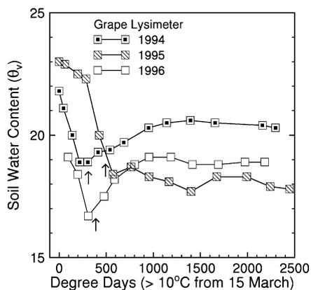
Fig. 2. Soil water content (expressed as percent by volume:  $\theta_v$ ) measured in the lysimeter during each growing season of the study. An individual data point is the mean of two access tubes measured at six depths (from 0.23 to 1.65 m below the soil surface). Arrows indicate approximate dates of the first irrigation each season (see Table 1 for calendar date of first irrigation each season).
