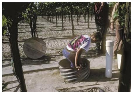
**Left and center, construction of the two large weighing lysimeters at KREC began in 1986. Each lysimeter consists of an underground chamber that houses a balance-beam weighing system with a rectangular “flower pot” measuring 6.5 feet wide by 13 feet long by 6.5 feet deep. Right, researchers enter the completed lysimeter.**
