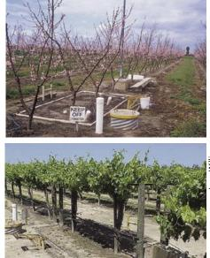
The Kearney lysimeters have been in constant use since 1987. One lysimeter measures water use in peaches, *top*, the other 'Thompson Seedless' grapes, *bottom*. The lysimeters have provided more accurate evapotranspiration values for peach trees and grape vines, information necessary in irrigation management decisions that ultimately affect plant health and fruit quality.
